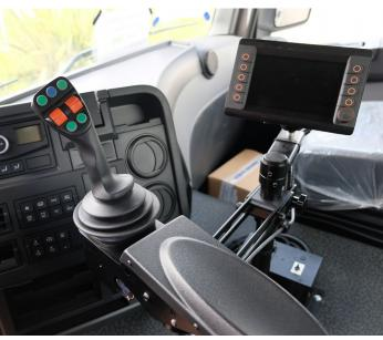
Joystick with screen and automatic dosage control
